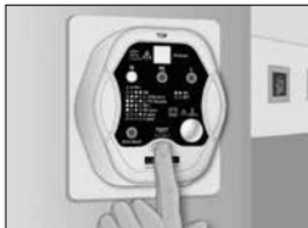
3. The line-side FI/RCD circuit breaker trips when the „TEST“ button is pressed (3 seconds).
